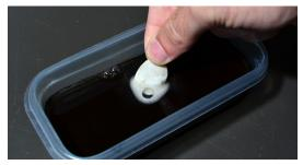
no reaction, the solution is expended. This test should be performed near the end of the recommended circulating time. If near the end of the recommended cleaning time the solution has been expended, more **RYDLYME** will be required to complete the job. However, if the solution is still active at the end of the recommended time, all the scale has been dissolved within the application and it is ready to be water flushed and returned to service.
